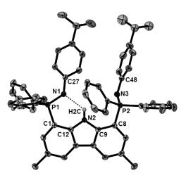
**Figure 2.** Thermal ellipsoid plot (50% probability) of  $\text{HL}^{Pipp}$ (**4b**) with hydrogen atoms (except H2C) and solvent molecules of crystallization omitted for clarity. Selected bond distances (Å) and angles (deg): P1-N1 = 1.574(2), P2-N3 = 1.575(2), N1-P1-C1 = 105.3(1), N3-P2-C8 = 106.8(1), C27-N1-P1 = 128.8(2), C48-N3-P2 = 127.0(2).
